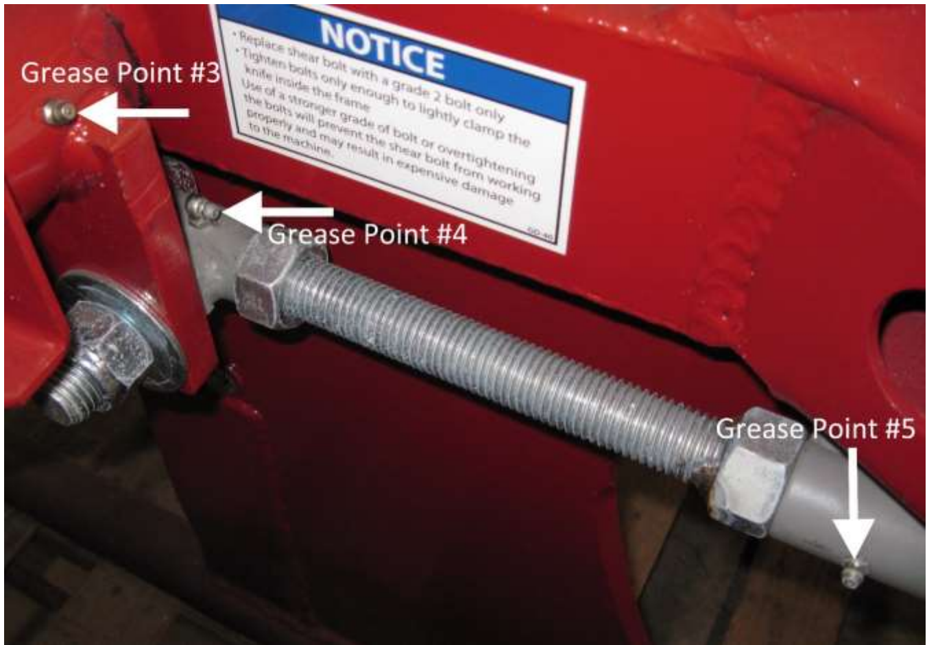
Figure 17: Grease Points on Packer Wheel Adjustment Rod
